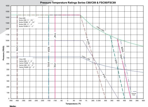
The practical pressure-temperature rating of a valve is determined by the limitations of the body material and seat/ seal material. The valve body ratings are based on ASME B16.34 rating for materials. The graphs are based on laboratory testing and our experience in the field. The seat ratings depend on the material, design, application, and function.
